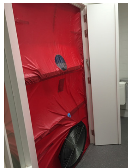
Figure 1: Blower-door with fan fitted in a lab door opening
